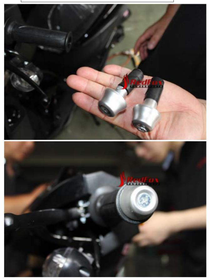
tips: Push the handle bar in hard to engage and screw it the end screw to tighten it
