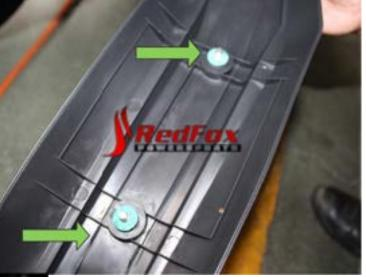
tips: Insert rubber first as shown in the picture and then insert the bolt with spacer on the back before installation
