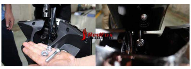
tip: best to remove the front panel to gain better access with tool to install the handle bar bolt and nuts.
