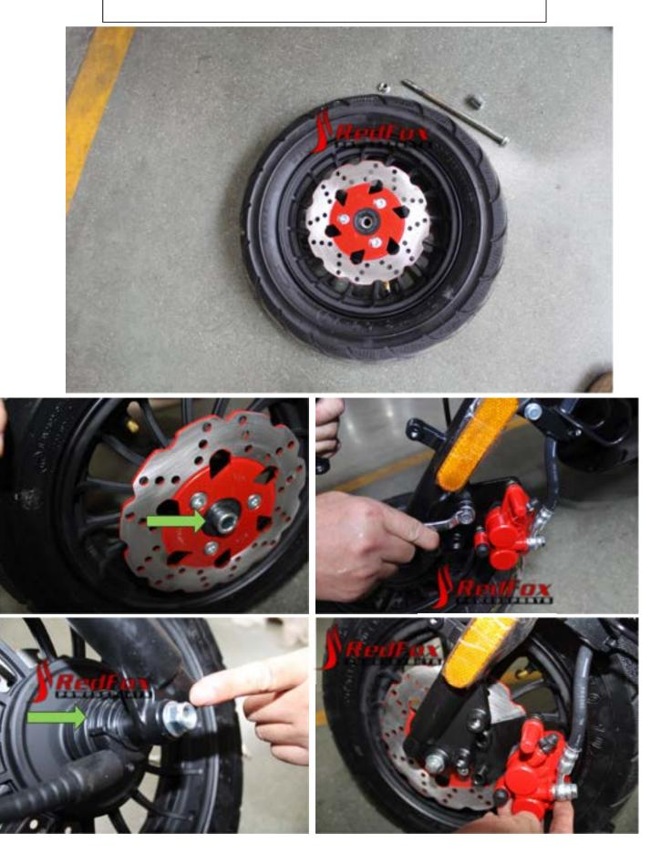
Tip: Remove brake caliper for easier installation on the front wheel, insert brake caliper after wheel is properly installed
