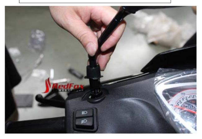
Tips: to screw in the mirror, make sure to connect the thread properly and thread in. Once it reach to a position you like, lock it down with the bolt on the miror turing it the opposite way to tighten it
