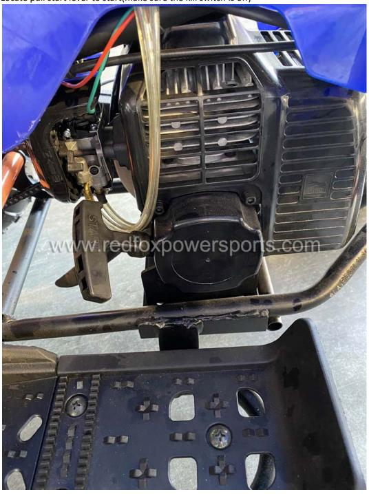
16. Locate speed limiter screw to adjust the throttle level
