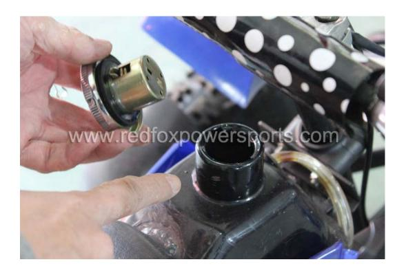
9. To shut off the ATV (press the red kill switch button or remove the kill switch strap cap to shut off)
