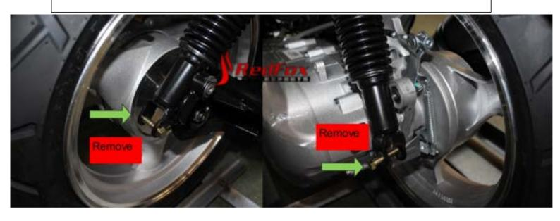
tips: It's best to have 2 person align the both right and left side shock together for proper and easier installation
