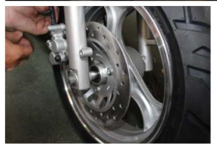
tips: Insert the front axle bolt from disc brake side for easier installation
