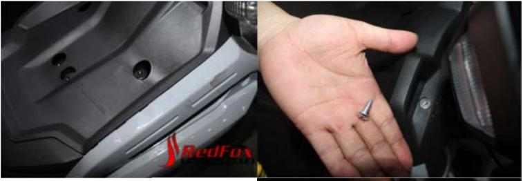
tips: semi clip in the plastic piece and then tigthen with the top 2 screw. Once screw is tighen, you can go back to clip in the plastic properly alot eaiser.
