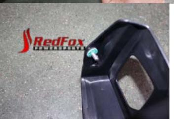
tips: pre-install the bolt with spacer and the paper spacer on the muffler for easier installation. Make sure the paper spacer goes to inside to protect the muffler high temperature
