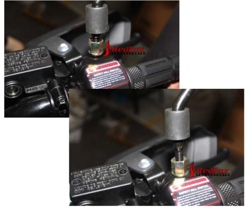
tips: Thread in the mirror first and secure with the gold bolt by turning the opposite way to lock it down to the position you want
