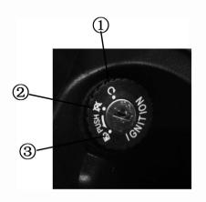
③ LOCK position Turn the switch all the way to the left, push it down and turn it to the LOCK position; the key can be pulled out. In this case, the vehicle can not be steered and the engine as well as the lighting system will not work.
