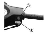
Engine stop off 5Turning the switch to this "X" position to power off, and checking the switch on "O" position before starting.
