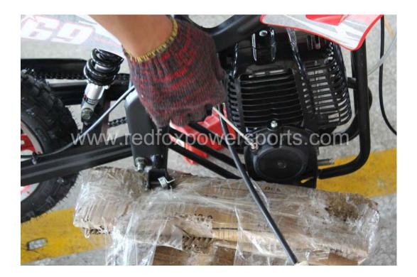
14. To shut off the engine simply locate the kill switch button or remove the kill switch strap cap
