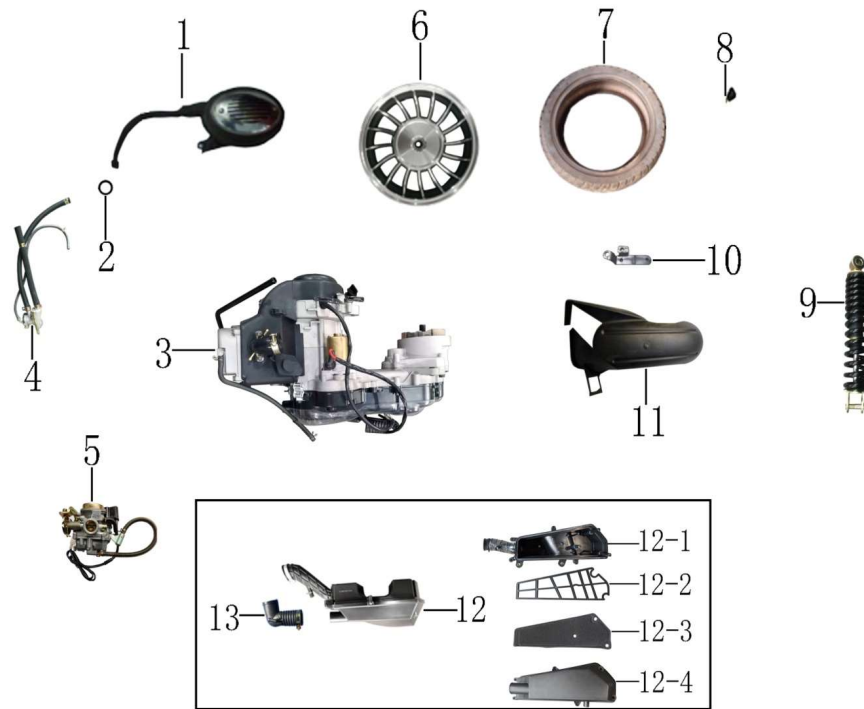
图8 发动机、化油器、消声器、空滤器、后轮及后减震 Engine, carburetor, muffler, air cleaner, rear wheel, rear shock absorber
